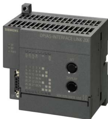
Figure 4-30 DP/AS-Interface Link 20E
