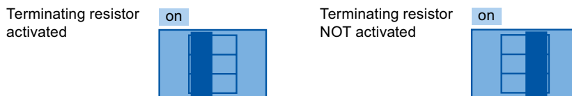
Figure 4-3 Setting of the terminating resistor
