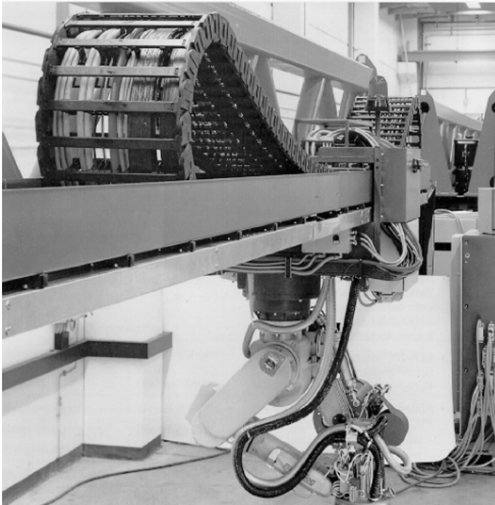
Figure 7-10 Example of using the glass fiber optic trailing cable in a drag chain
